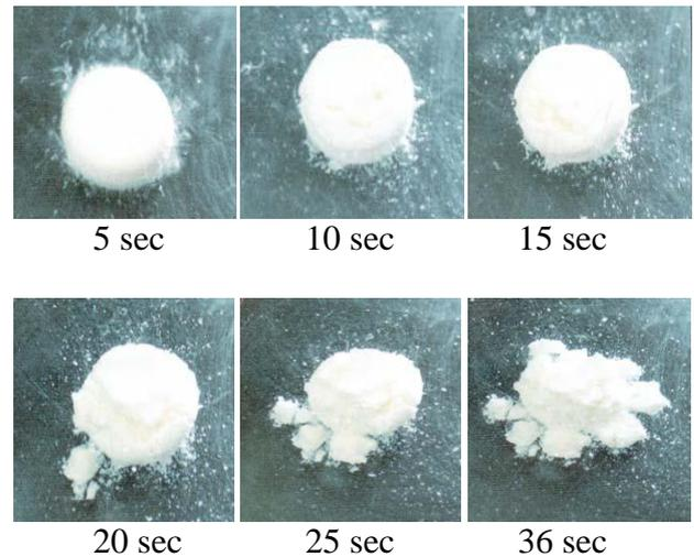
**Figure 2: Disintegration process of tablet (F-2).**
